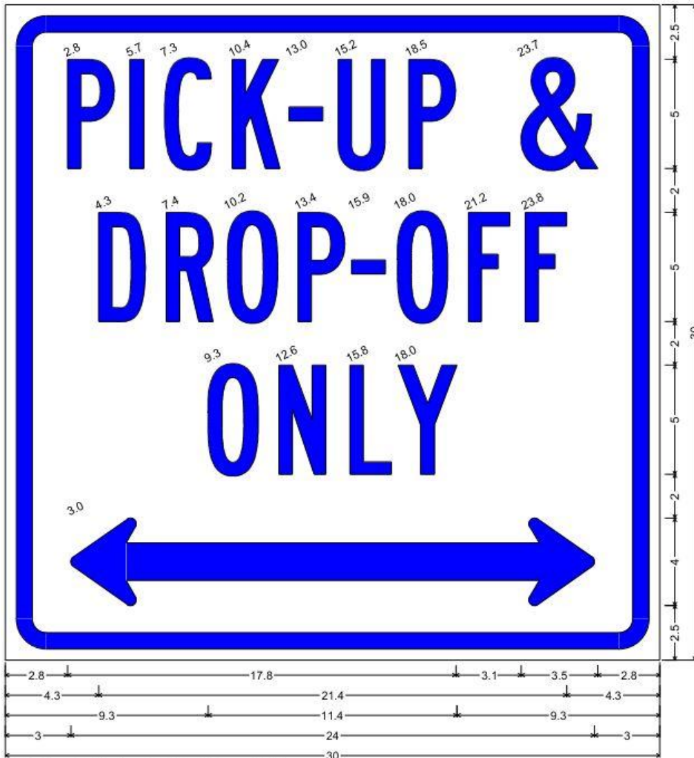
1.9" Radius, 0.8" Border, 0.5" Indent, Blue on White; "PICK-UP &" B 2K; "DROP-OFF" B 2K; "ONLY" B 2K; Double Headed Arrow Custom - 24.0" 0";
