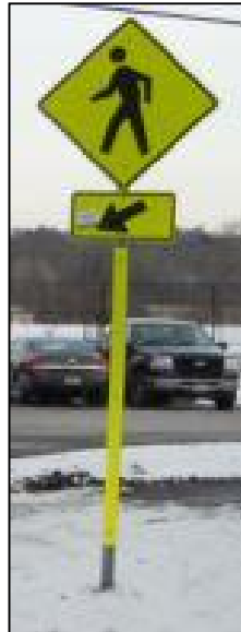
RETROREFLECTIVE TAPED POST (PLACED ON S1-1 POST)
