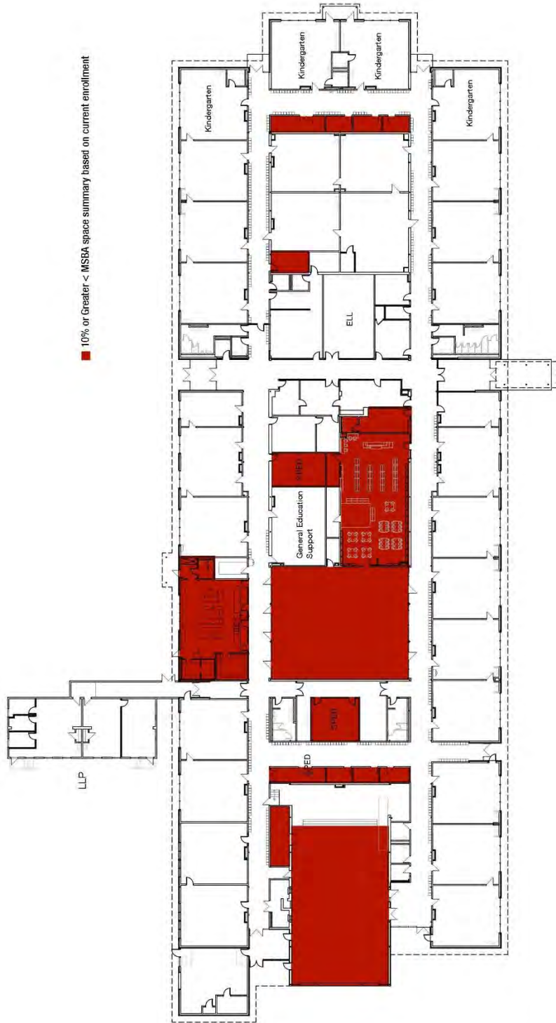
Bowman Elementary School First Floor Deficiencies (Per MSBA Requirements)
