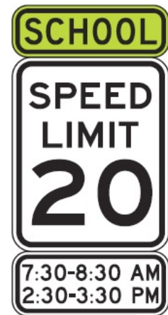
Fig. 9-4: R2-1 Sign with S4-3P and S4-1P Plaques (Source: MUTCD)
