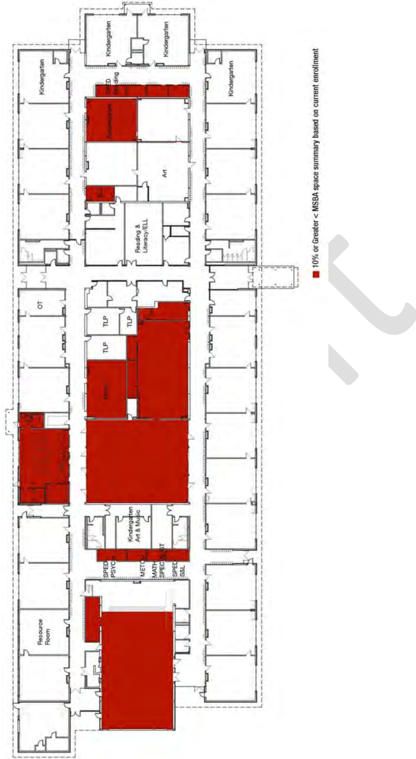
First Floor Deficiencies (per MSBA Requirements)
